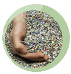
**Our closed loop manufacturing drastically reduces waste**. We're not new to the game. We were in recycling long before it came into style. In 1993 we developed a patented technology that takes recycled plastic and combines it with post-production wood waste from our wood manufacturing facilities. This new composite material is injection molded and utilized in everything from panel frames to chair components. It's not pretty to look at, but it's very strong and it's inside where it counts.
