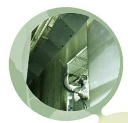
Our powder-coat paint process reclaims up to 99% of the overspray with minimal discharge to the environment.
